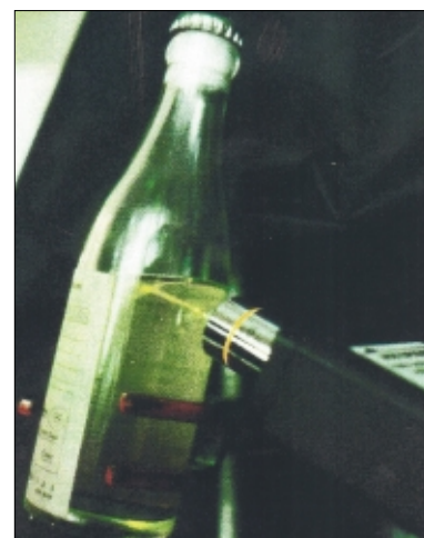
Figure 4. Raman analysis of process grab sample inside sealed sample container.
